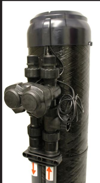
*Finally place the cap on the tank, ensuring that the wire connections are in the wire trough as shown.*
