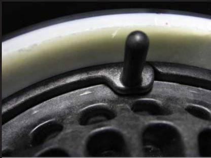
*Working clockwise, push the retaining ring into the groove until the end snaps into place. Gently pull on lid assembly to seat o-ring.*
