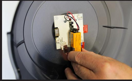
*If desired, connect a 9 volt battery to DROP Board. The battery allows the filter to monitor water flow during a power failure.*
