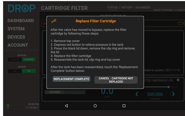
*After filter cartridge is installed, double check that the top snap ring is installed properly and then press the "Replacement Complete" button in the app. The motorized bypass will begin to open and your cartridge filter will begin to fill with water. As it is filling gently press the red button on the top of the tank to bleed off air in the tank as it is filling. Once water begins coming out of the pressure relief button, you can release it.*
