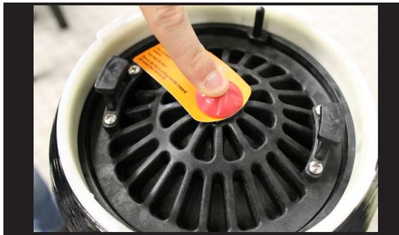
Remove top cover and relieve pressure in tank by pressing red button.
